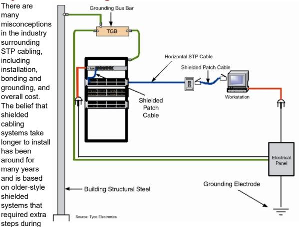
installation. Many of todays shielded components include die-cast metal jacks that no longer require special bonding of the shield, making the installation time comparable for both UTP and STP. STP systems really only require a little extra time to separate the overall shield from the cable. In addition, STP systems do not typically need to be tested for ANEXT, which can be a fairly time-consuming process with UTP.
