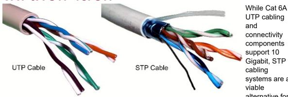
alternative for running 10 Gig over copper. As shown in the graphic below, the shield in our STP plenum and riser-rated cable does an excellent job of eliminating ANEXT, providing an improvement in ANEXT performance over Cat 6A UTP.
